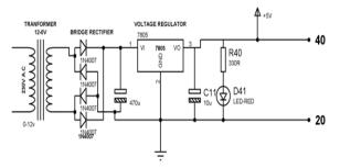
Transformer is static device which transfer electrical energy from one circuit to other circuit with change i n voltage or current without change in frequency. In this step down transformer is used. Usually, DC voltage s are require d to operate various electronic equipment and these voltages are 5V, 9V or 12V. But these voltages cannot be obtained directly. Thus the a.c. input available at
